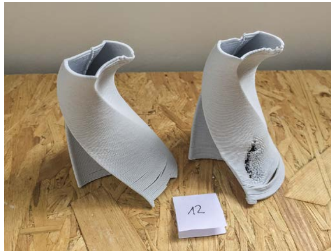
Figure 1: Porcelains printed in a DeltaWasp 20 40 Turbo2 3D-printer showing typical defects
